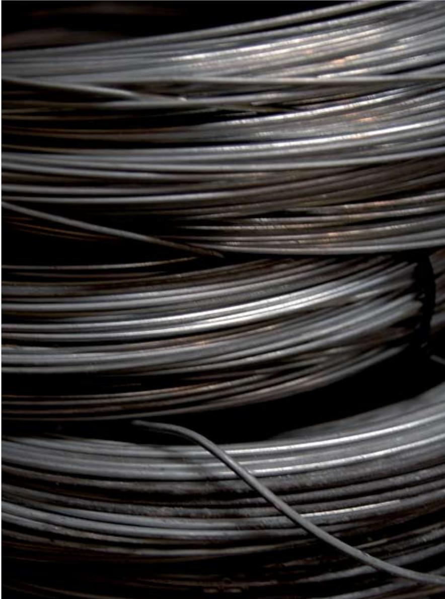
input in Transvaal Gate's production of commercial chain link fencing.
